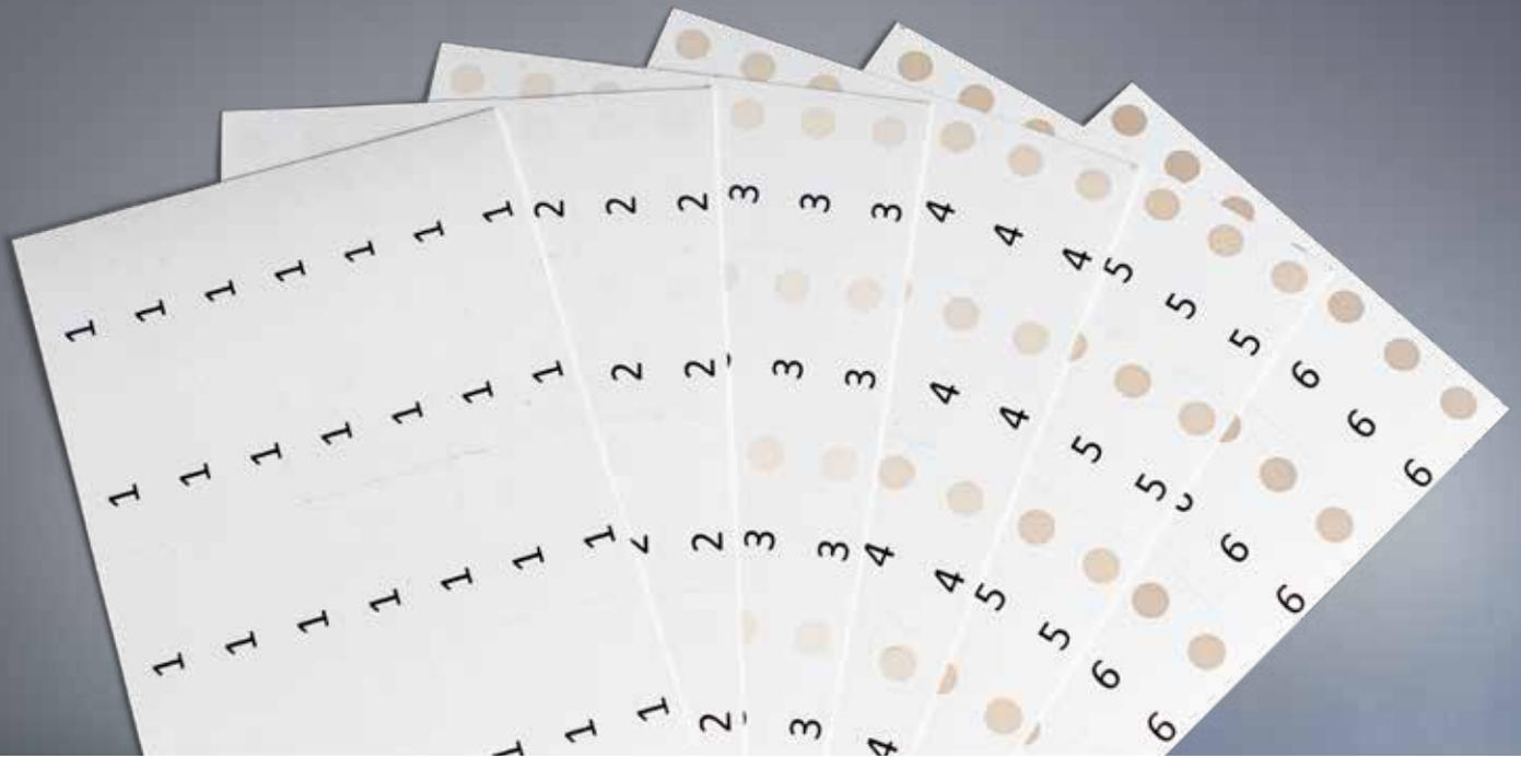
The so-called plasma indicators are a very reliable and economic method of proving the success of a plasma treatment. The indicators are added to the running plasma process and reliably show the success of the plasma treatment.
